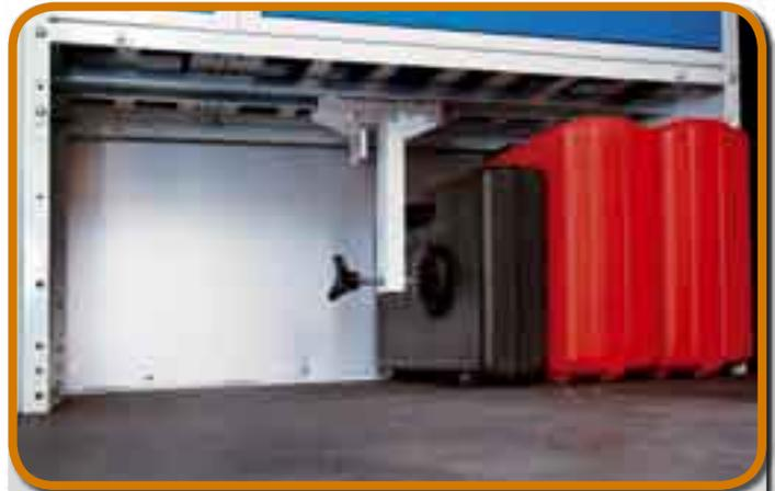
Syncro tool box secure system can be installed on open wheel housing covers. The grip shuttle moves in one direction only. Once it comes in contact with the tool box, this system secures the tool box in place. By turning the rear flywheel, the disc is further tightened up against the tool box for additional safety. To release simply press the locking lever.
