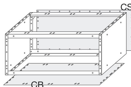
To close off an additional rear angle is installed together with a closure panel, this can be fitted to the top, bottom or rear of the wheel housing cover, depending on requirements.
